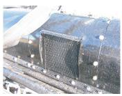
**Hydraulic Cooler**-Equipped with removable debris screen. Located within easy sight of the operator
